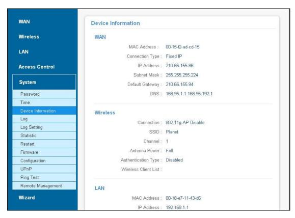
**WAN:** This field displays the WRT-415 WAN interface MAC address, DHCP client status, IP address, subnet mask, default gateway and DNS. Click "DHCP Release" to release IP addresses get from ISP for the WAN port. Click "DHCP Renew" to get a new IP addresses from ISP for the WAN port.
