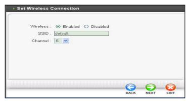
You can either enable or disable the wireless interface. If the Wireless LAN is enabled, you should set a ESSID and Channel for the wireless client to access. Click "NEXT" to continue.
